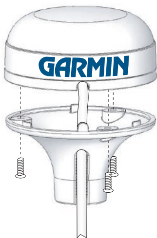
Attaching the Pole Mount to the GPS 17
